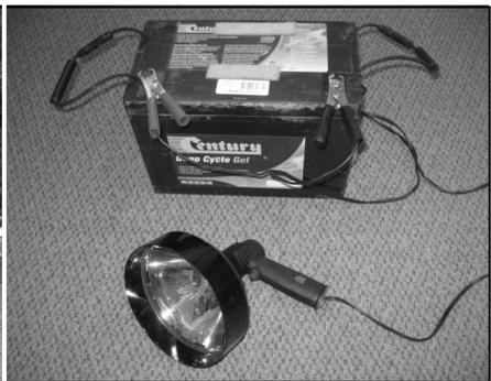
**Figures 1–2.** Equipment used for crocodile survey: 1. Boat with a 30 hp engine; 2. Spotlight (100 W) connected to a battery (12 V, 100 A);
